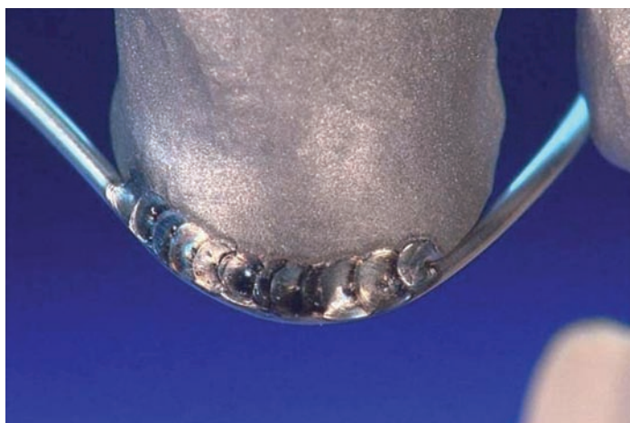
Figure 7 — The welding in micro spaces have been optimized; correction of the edges with the help of a thick wire 0.35 mm
