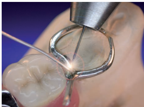
Figure 2 — Area of heat influence reduced - repair of a bridge with clasps without the need to disassemble the resin saddles
