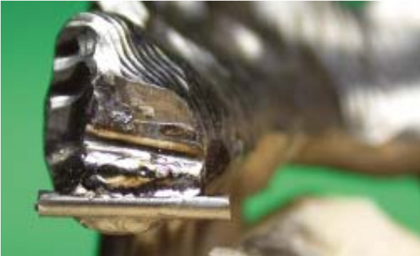
Fig. 32 and 33: one wire is welded to the lower groove of the one piece; the other wire-pin is welded to the upper groove of the other piece.
