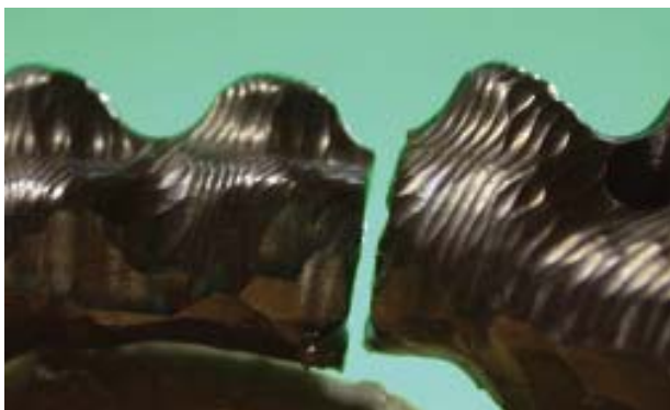
Fig. 29: after the cut a step of more than 1 mm was created between the two pieces.
