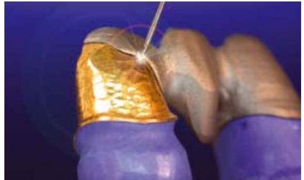
Fig. 12: the first tacking impulse is always directed to the area where the gap between coping and bridge element is the smallest.
