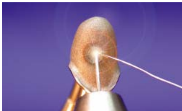
Fig. 3: Depending on the surrounding material thickness, the hole can be closed with one phaser impulse.
