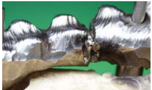
Fig. 34: it is sufficient to place two connecting pulses lingually (between each wire pin and the other side) to further stabilize the correct position.
