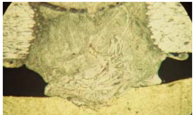
Fig. 16: when this welding task has been performed properly, the cast metal has nicely fused with the Gold copings (metallurgic cut, Hellfeld, 100x magnification).
