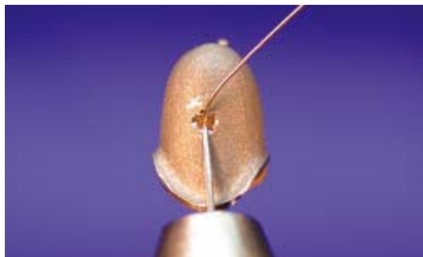
Fig. 2: Hole in semi precious alloy crown. The welding wire is placed into or over the hole.
