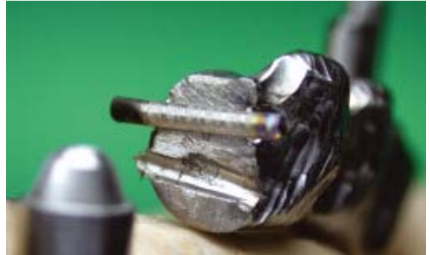
Fig. 32 and 33: one wire is welded to the lower groove of the one piece; the other wire-pin is welded to the upper groove of the other piece.
