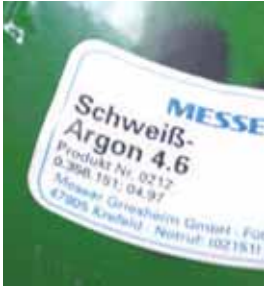
Fig. 1: Successful welding requires Argon with a purity of 99.996% or more.
