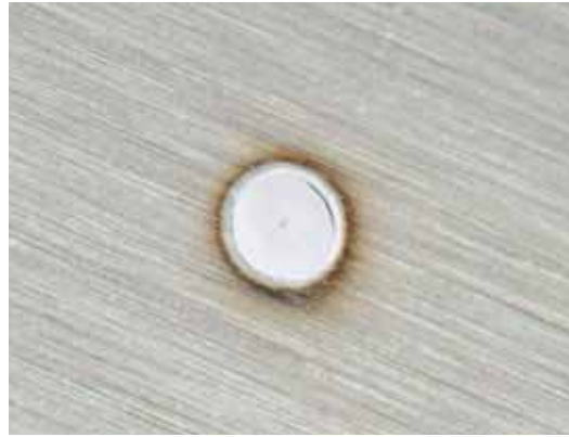
Fig. 3: Shiny, silver welding spot on Titanium indicates correctly adjusted Argon gas.
