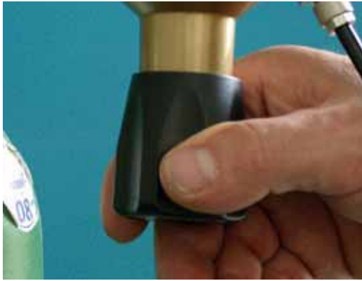
Fig. 2: The gas flow rate is adjusted with the valve on the bottom of the gas regulator. The actual flow rate is shown on the right gauge.
