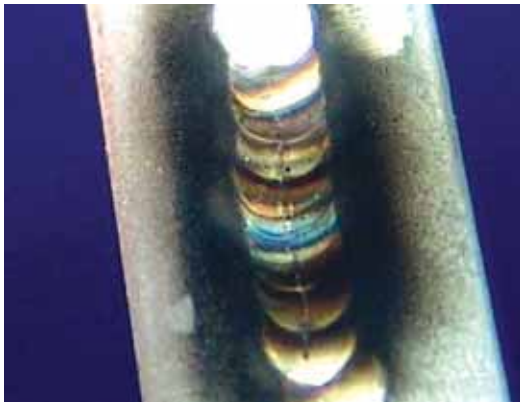
Fig. 4: Illustration of the worst case. Blue and yellow discoloration at the welding spots, heavy soot and micro cracks in the spots (causes and countermeasures for cracks will be discussed later).
