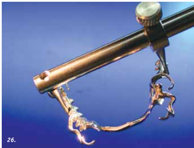
Figs. 24, 25, 26: Once the “ring is closed”, even cases that tend to distort easily can be welded with ease.
