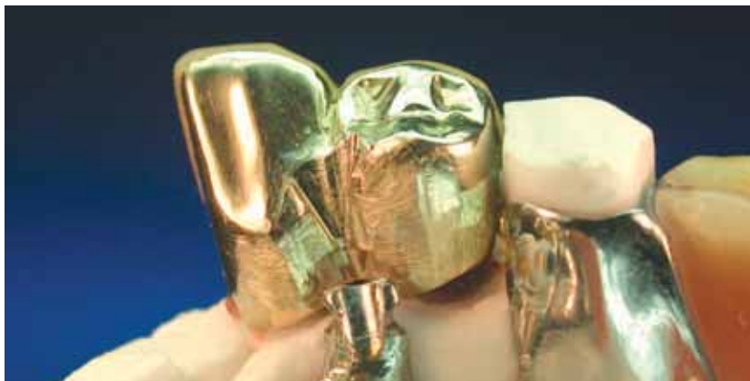
Fig. 6: Inadequately soldered telescopic crowns broke off the partial. The old solder material was completely removed and the case prepared for welding.
