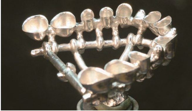
Fig. 13: ...and after the casting process. A minimal amount of finishing was needed
