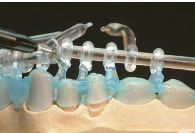
Fig. 10: The casting object and the volume rings are connected with Metablu using the "cold" application method
